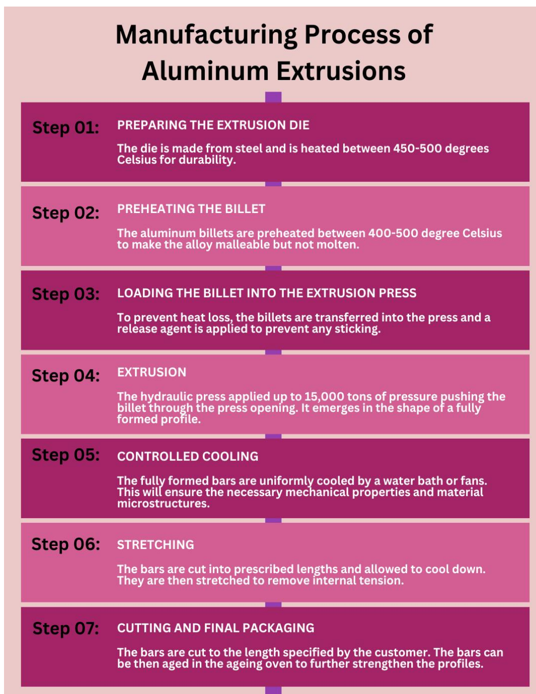
Figure 17: Manufacturing process of aluminum extrusion
